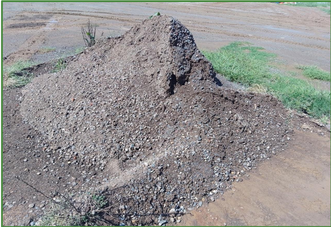
Photograph 3: Closeup of small road base stockpile (location in photograph 2 above)
